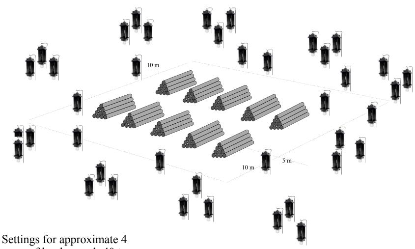
Settings for approximate 4 acres of lumberyard -40 traps total (10 traps single, 30 traps in 10, 3-trap clusters), Total of 20 lures.
