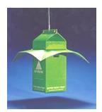
According to STS protocols- Milk Carton traps shall be used where a previous year's trap locations caught 5 or more male moths. Each trap will contain an approved pheromone lure and a 1-inch by 4-inch dichlorvos pesticide strip (registered as Vaporlure II).
