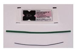
Prepare the lure and DDVP strip for installation; Vaportape (DDVP strip), Disparlure (lure string) and 7 inch twist tie.
