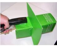
Open hood and then insert and staple to trap body making sure all four hood tabs are tucked inside the perforations of the trap body
