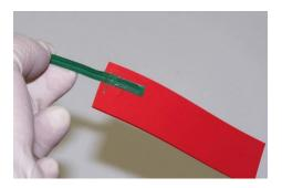
Attach Vaportape to twist tie with staple pliers
